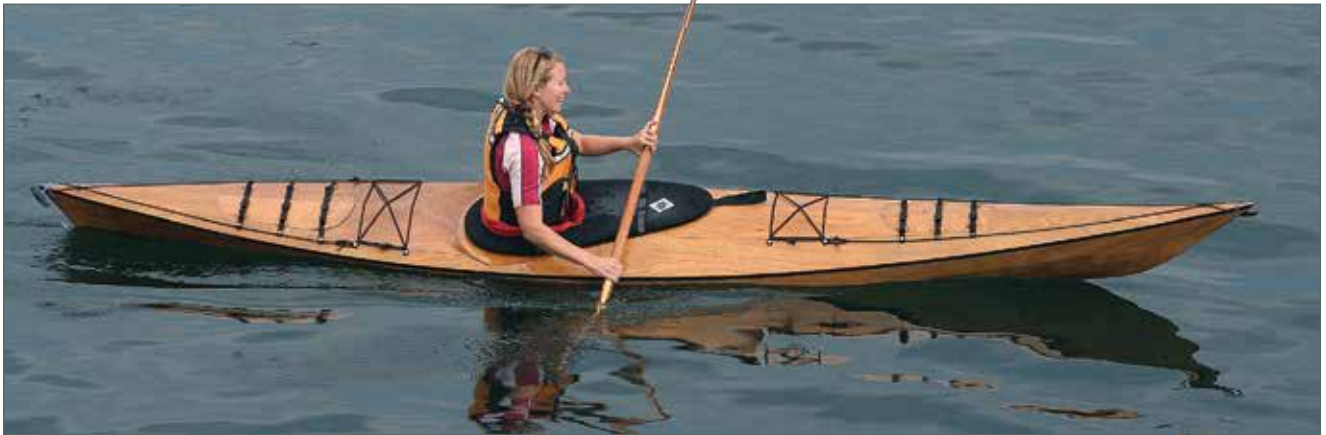
The Pinguino turns nicely when heeled to one side, or "edged"; in this position, it will continue to turn even when the paddling stops.
