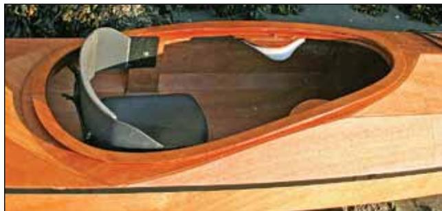
**Above**—The adjustable backrest and thigh rests, together with options for the seat, make the Murrelet easily custom-fitted to the user. **Left**—Blocking under the stowage compartment bands puts pressure on the edge gaskets to help keep water out.
